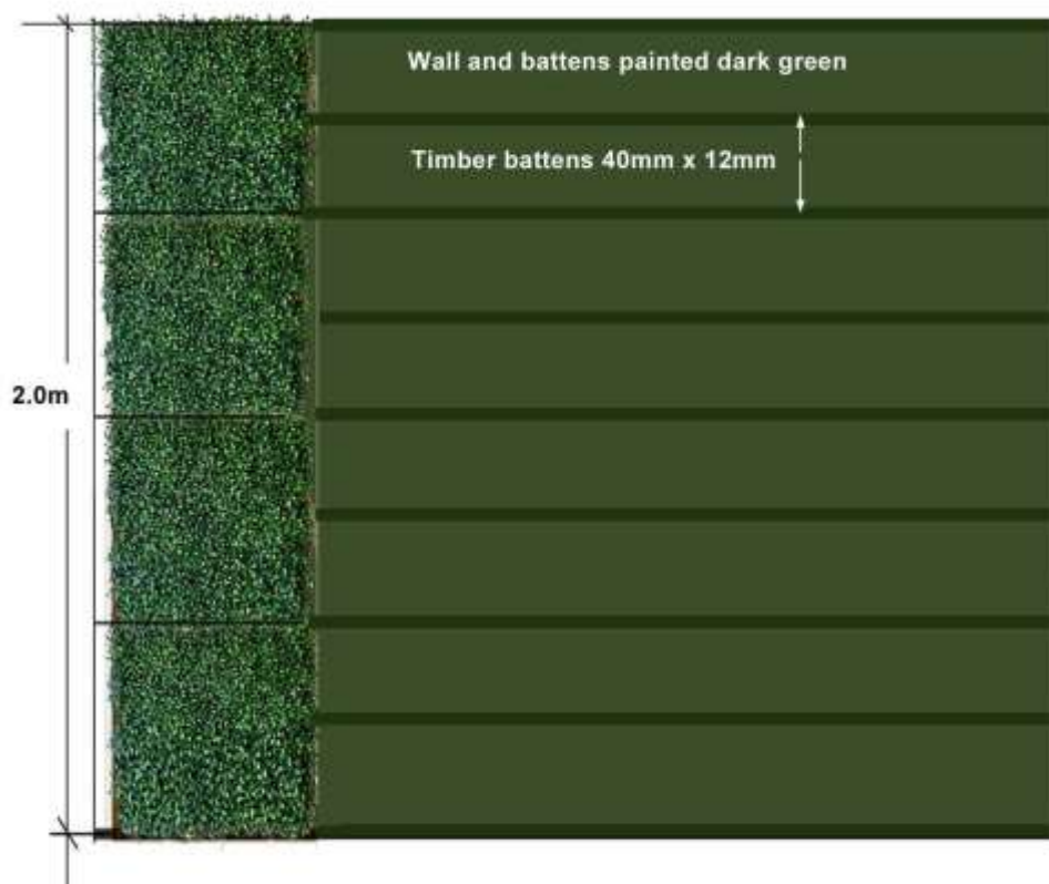
Fixing Readyleaf to a solid wall (option 1)
