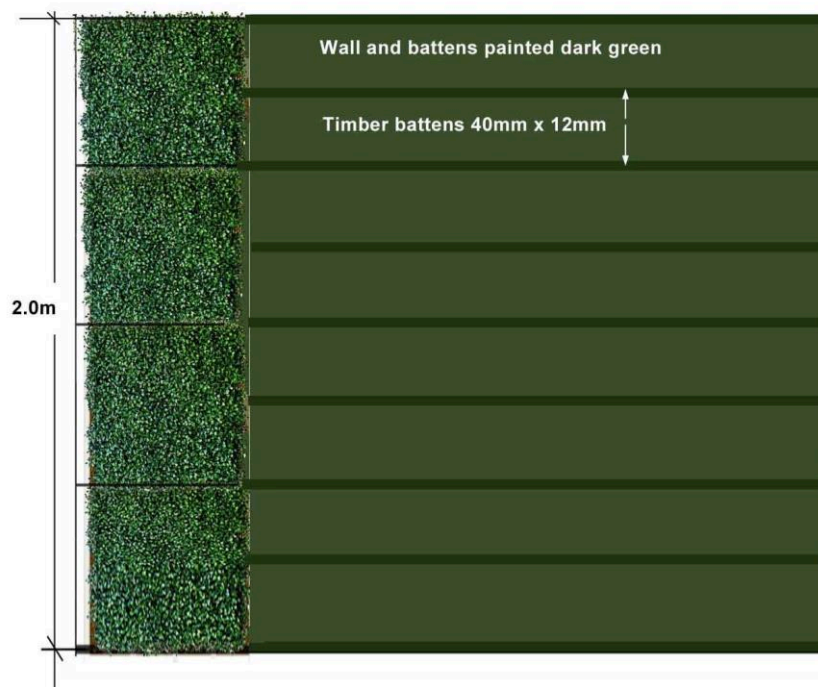
Fixing Readyleaf to a solid wall (option 1)
